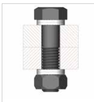
Hexagon bolt in a through-hole, secured on both sides
