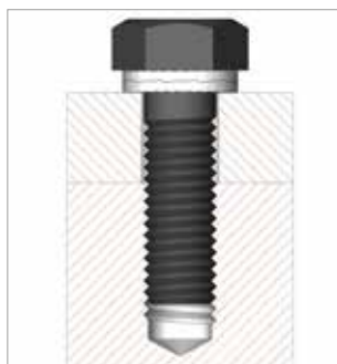
Hexagon bolt secured in a blind hole
